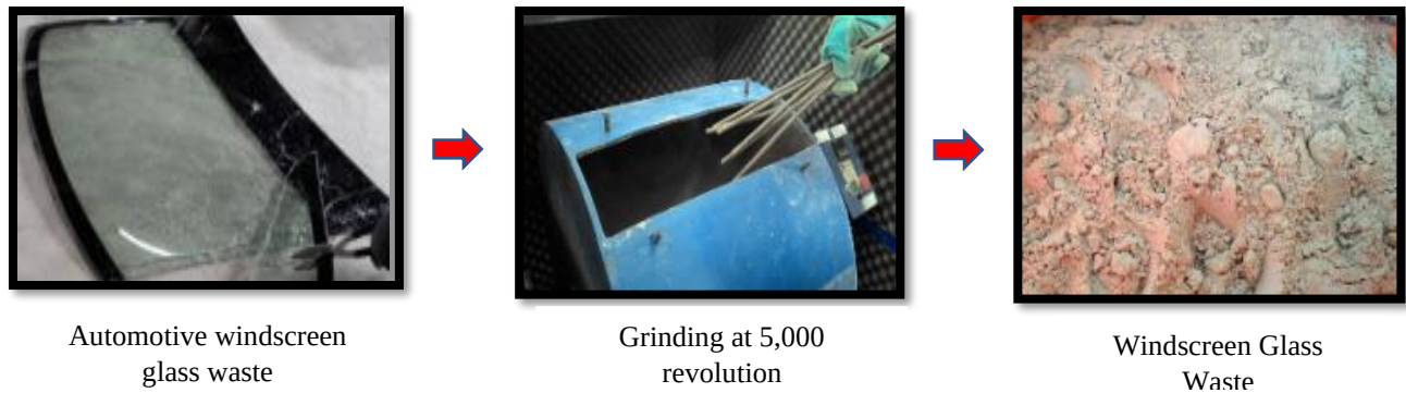
Figure 1. Preparation of automotive windscreen glass waste (WGW)
