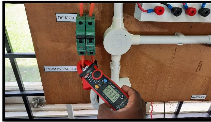
Figure 1. Photovoltaic current measurement
