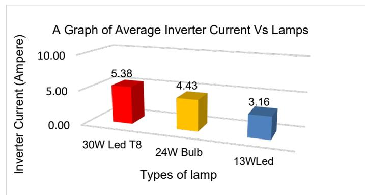
**Figure 3.** Graph of Average Inverter Current
