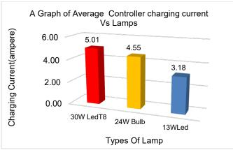
Figure 4. Graph of Average Controller Charging Current
