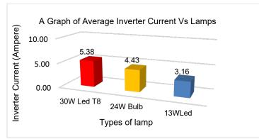
Figure 3. Graph of Average Inverter Current
