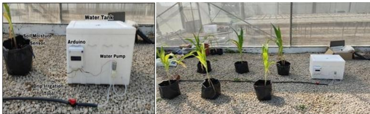
Fig. 5: The implementation of automated drip irrigation system
