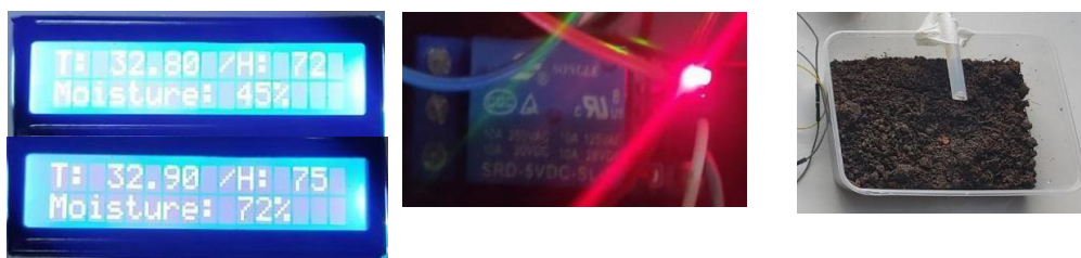
Fig. 6: LCD, relay and water pump output when the soil is wet
