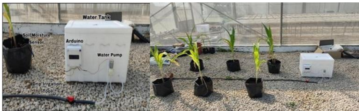
Fig. 3.1: The implementation of automated drip irrigation system
